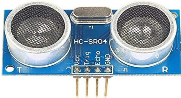
Figure 47: SainSmart HC-SR04 ultrasonic transceiver
